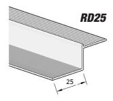
With the increased requirement for acoustics and the use of 15mm plasterboard, Type RD Reveal trims are used to create horizontal or vertical reveal details within areas of dry lining, suspended ceilings, door frames, skirting and windows frames and many other architectural features.
