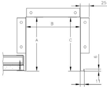
Manufactured from Steel or Aluminium, safety edge c/w j channel. Joining plates and can be powder coated any Ral colour.
