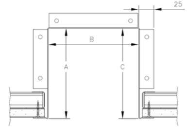
Manufactured from Steel or Aluminium, taped edge x 2. Joining plates and can be powder coated any Ral colour.
