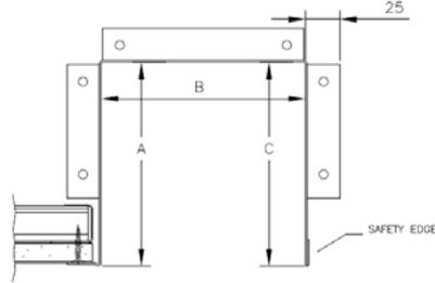
Manufactured from Steel or Aluminium, safety edge and taped edge. Joining plates and can be powder coated any Ral colour.
